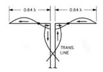
wavelength per side. The formula to determine the length of each side in feet is 599 divided by the frequency in MHz.
